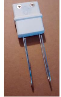
If instead you see blinking Orange followed by blinking Blue, this indicates that you may need to tighten the stainless steel screws a little bit tighter. Do so, and then repeat this test.
